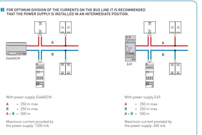
NOTE: If a UTP5 cable is used in alternative to the L4669 BUS cable, distances are halved.
