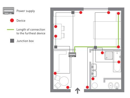
2 THE TOTAL LENGTH OF THE CONNECTIONS MUST NOT EXCEED 500 m (CABLE EXTENDED).
